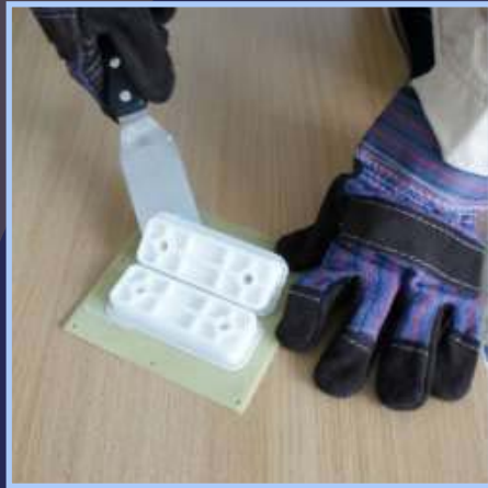
Removal of Component from AM Process - FDM
