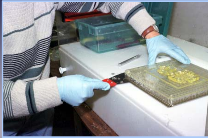
Removal of Component from AM Process SLA or SL (Pre Oven)
