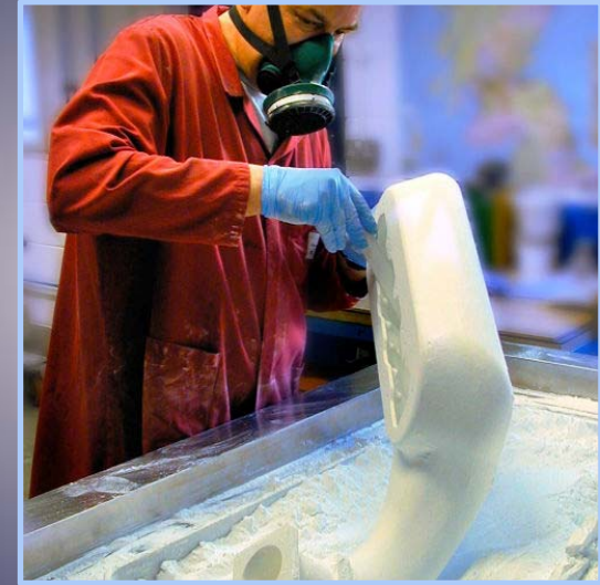
Removal of Component from AM Process – SLS
