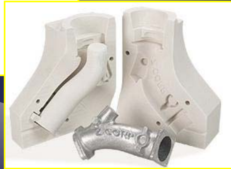
Example of investment metal casting using 3D Ink Jet Printer.
