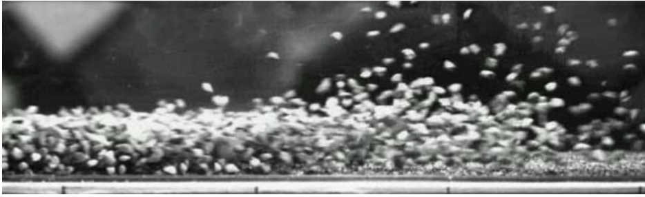
FIGURE 2.8: The head of an avalanche of gravel passing down an inclined chute. The flow is from left to right. At the head, particles saltate above the free surface, while behind in the body of the avalanche a dense flowing layer dominates.
