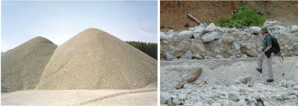
FIGURE 2.4: Polydispersity of granular materials. Left : A pile of well sieved gravel. This has a grainsize distribution that is composed of a small range of sizes, of the order of centimetres. Right : Detritus deposited after a debris flow. The grainsize distribution features every size of particle from clay to boulders, spanning over at least 6 orders of magnitude. (© United States Geological Survey)
