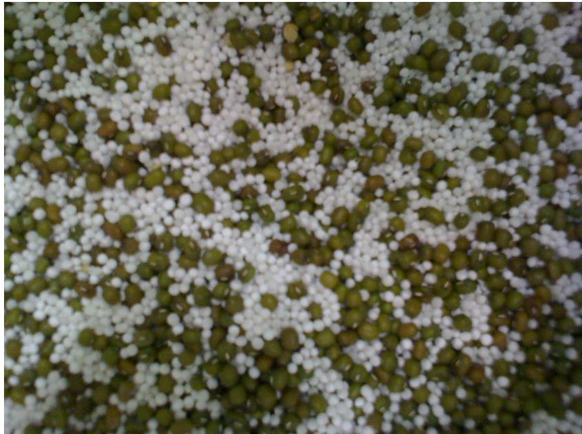
FIGURE 3.7: A mixture of mung beans (green) and tapioca seeds (white). The relative size ratio of approximately 1.5 will cause rapid segregation, and the sharp colour contrast will enable simple particle size distribution measurements by particle image velocimetry.
