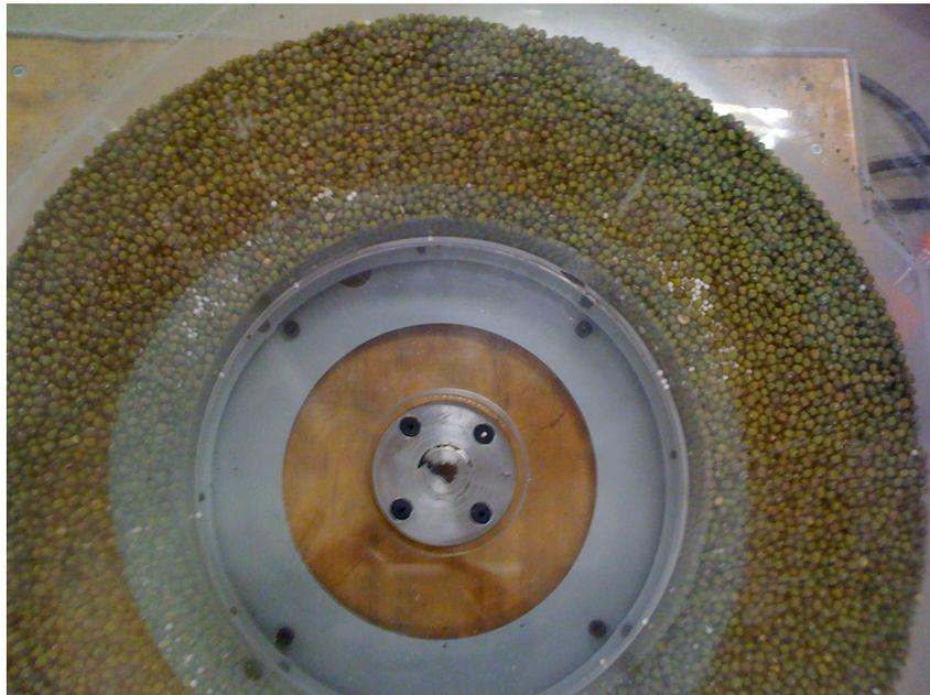
FIGURE 3.8: A top down view of the system after segregation. Mostly green particles are visible from the top, indicating that there is a high concentration of large particles there.
