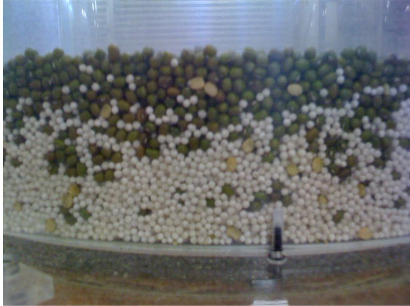
FIGURE 3.9: A side view of the system after segregation. There are noticeably two regions of differing particle size distribution. We see small particles at the bottom, and large particles at the top.
