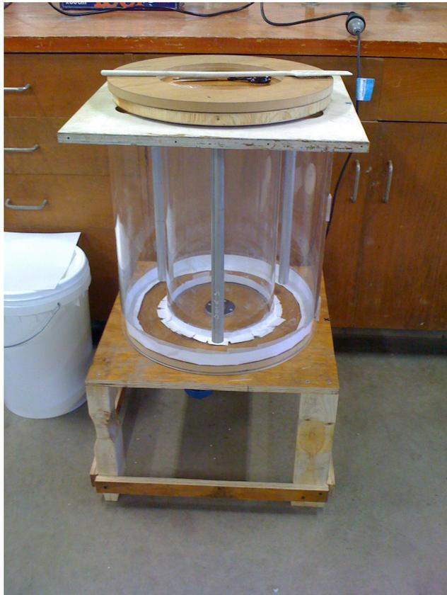
FIGURE 3.4: The shear ring apparatus after construction. Perspex walls are mounted on a wooden frame, which holds both the shear ring and the motor.
